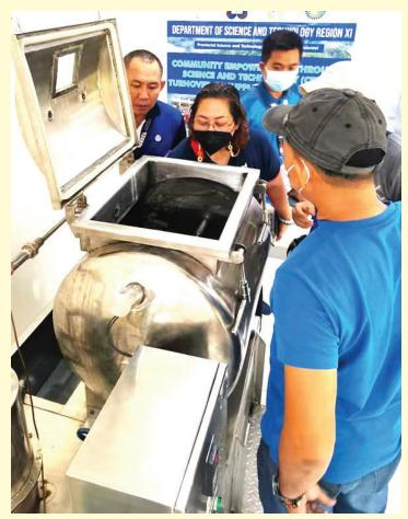
This vacuum fryer is a machine designed to fry vegetables, fruit, fish, and meat at low temperatures. This equipment has the capacity to reduce the oil content of the food. It can also help to inhibit the loss of nutrients that commonly occurs with food cooked or fried at high temperatures.
